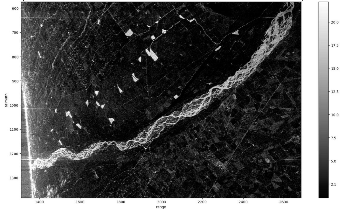
SWOT measurements of radar signal to noise ratio capable of observing complex rivers.
