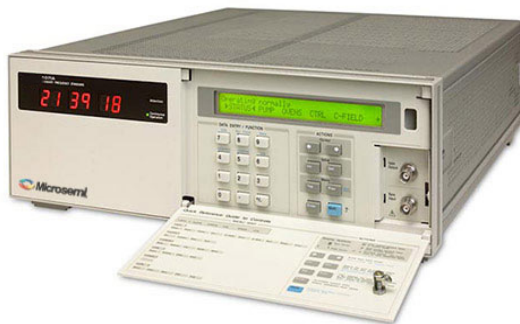
Cs Frequency Standard Microsemi 5071A df/f \sim 10^{-12}
