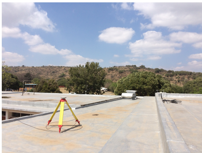
Figure 2. The GPS-702-GG Novatel dual-frequency antenna installed on top of the building at HartRAO. The 4380A timing system uses this GPS antenna to update the rubidium clock.
