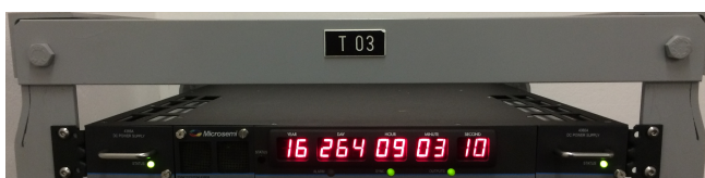
Figure 1. The rubidium 4380A timing system for the new LLR station at HartRAO. The system is currently being tested for short and long term stability against Hydrogen masers.
