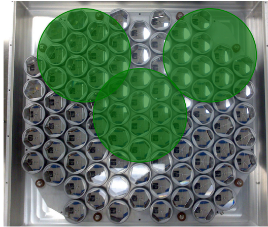
Figure 3 - Sketch of the intended multiple-CCR FFDP investigations of the Galileo IOV tray: the green areas are parts of the LRA lit with the expanded laser beam at 532 nm.
