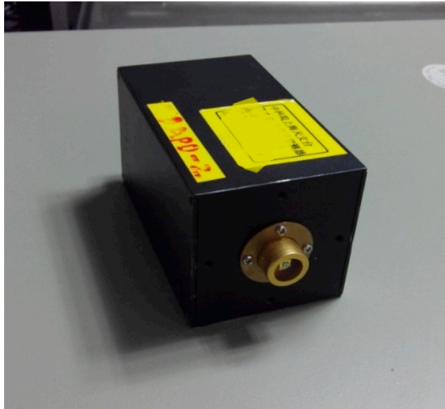
Fig.5.The Si- APD detector for detecting laser echoes
