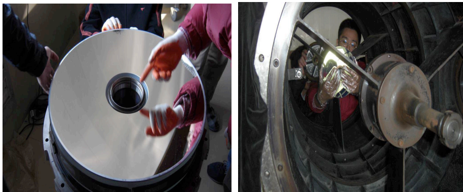
Fig.1 Installation of the recoated primary and secondary mirror
