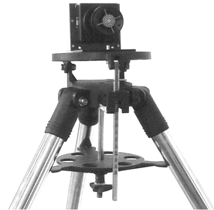
Fig. 2: The ELT detector package EM installed on a tripod in front of the WLRS telescope.
