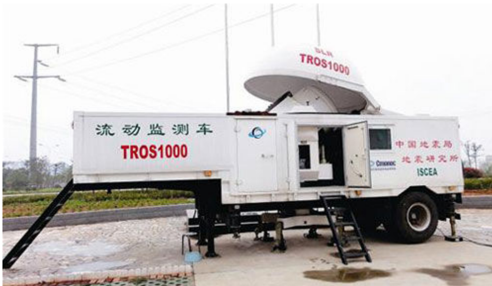
Fig.2 Chinese new mobile SLR system with 1-meter-aperture receiving telescope
