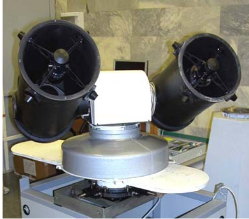
Figure 8. Miniature modular SLR station
