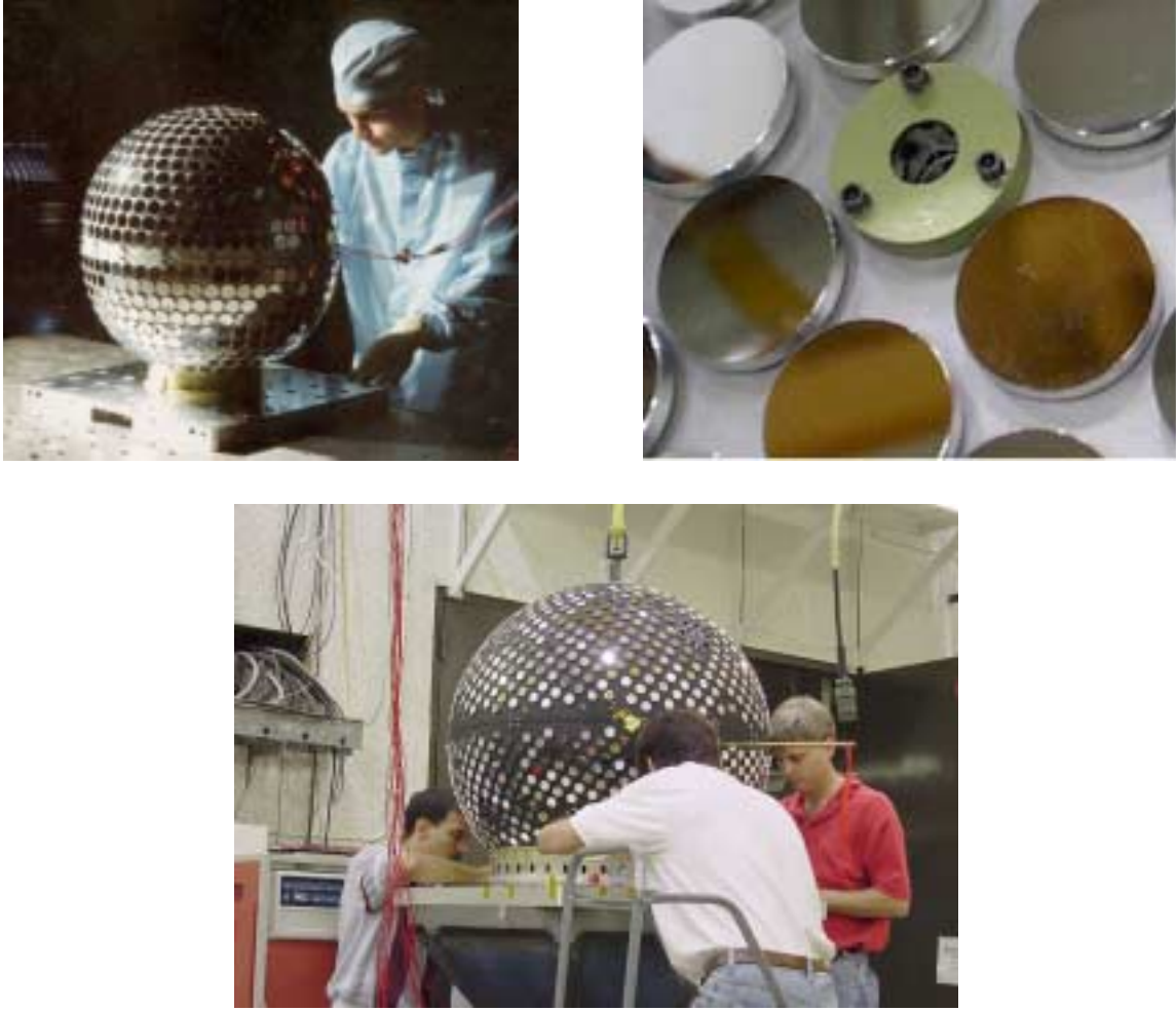
Figure 1: Starshine 1 (upper left panel). Individual retroreflector mounting on Starshine 2 and a few student-polished mirrors (upper right panel). Starshine 3 during vibe test setup (bottom panel).
