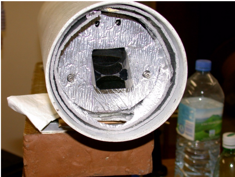
Figure 5: Thermal insulation of the right-angle prism and its adjusting mount
