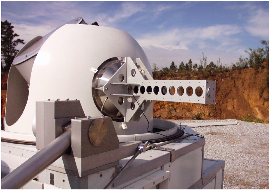
Figure 6: The support structure mounted at the elevation axis of the SLR telescope serves for the determination of the excentricity vector of the system invariant point with respect to the SLR marker.
