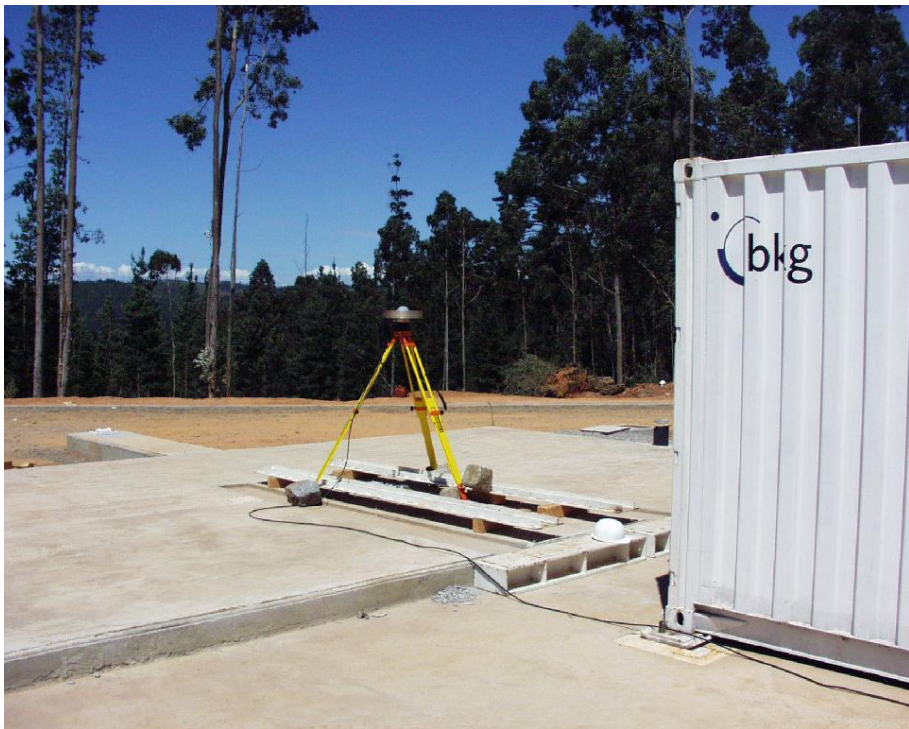
Figure 5: A GPS antenna located over the VLBI system reference point during the local survey.
