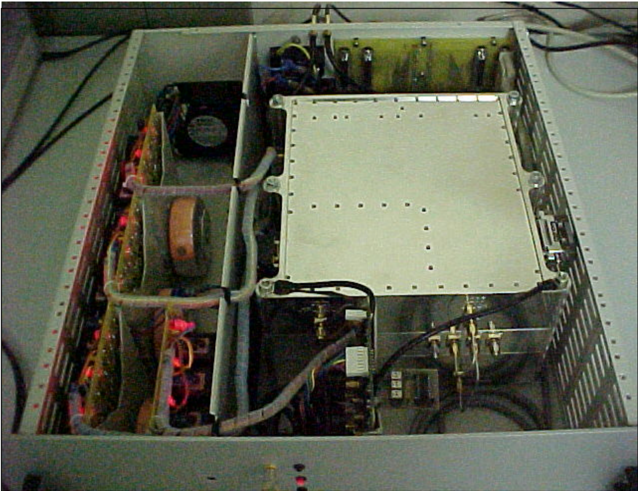
Fig. 3: 19" Rack Module, with 2 Event Timer Modules, Clock Module, Input Board, Power Supply
