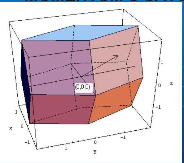
Possibilities of acccumulated momentum's saturation are exhausted when the momentum vector goes out of the figure of disposable kinetic momentum. At this time there must be procedure of desaturation of reaction-wheel system
