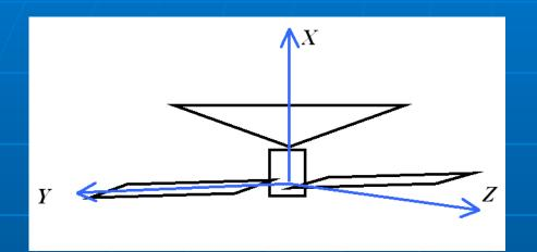
SC orientation relatively to the Sun is defined by two angles  $\alpha$  and  $\beta$  in the structural coordinate system (OXYZ)
