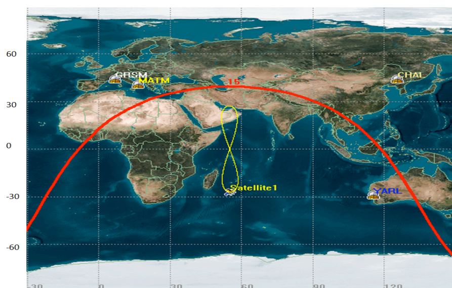
Figure 1: Visibility circle when the satellite at 27deg S latitude
