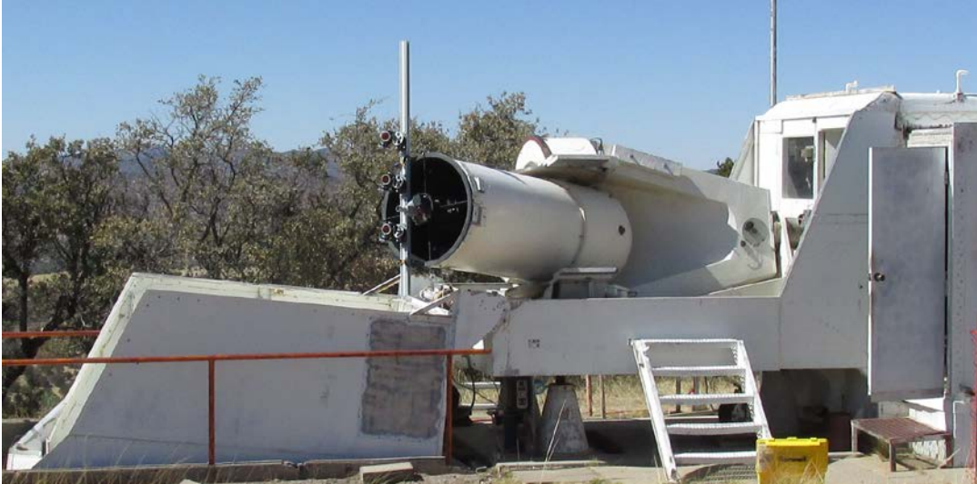
Figure 23. SLR w/target bar mounted vertically to the telescope. Attached targets were positioned as they scribed circles about the y axis.
