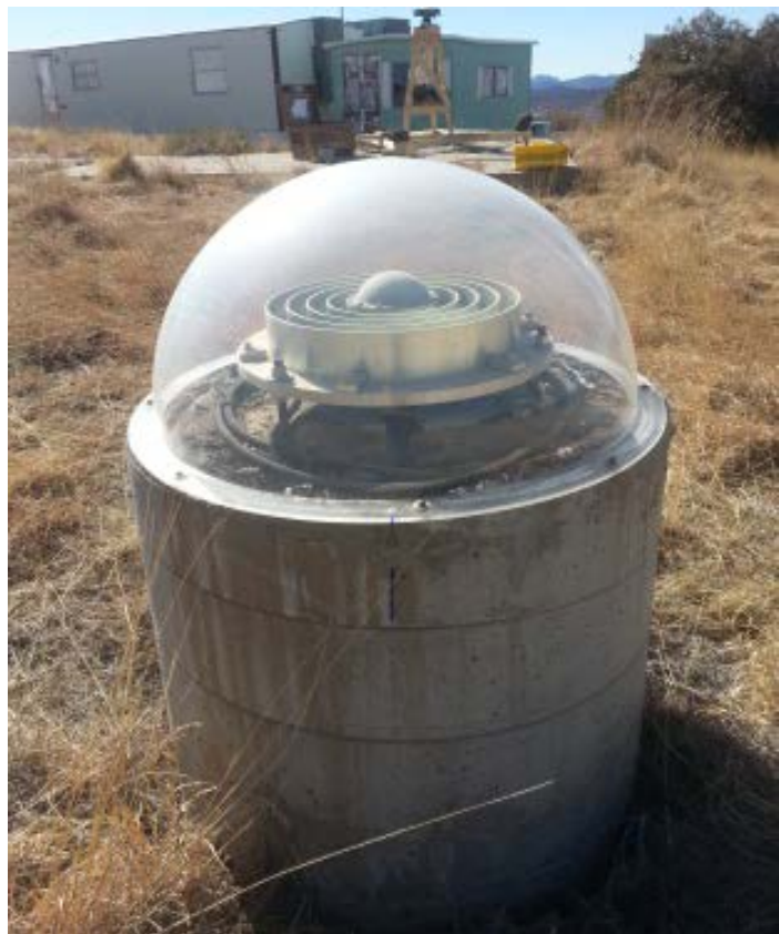
Figure 20: MDO1 w/choke ring antenna
