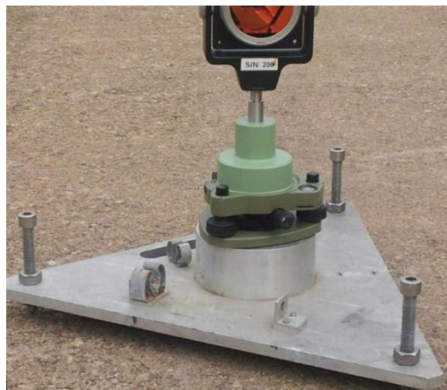
Figure 13: NGS trivet used on supplemental points
