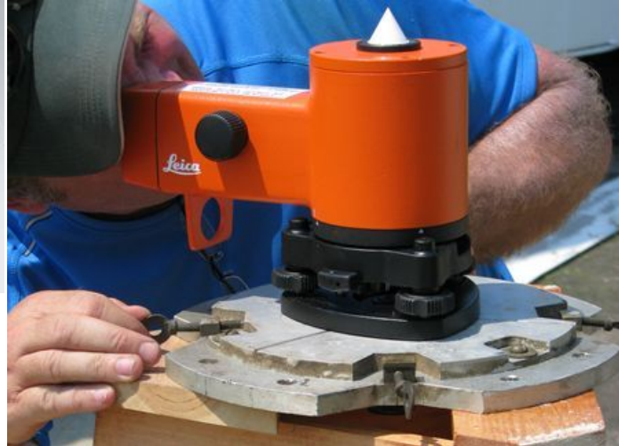
Figure 15: NL Collimator used to center the tribrach
