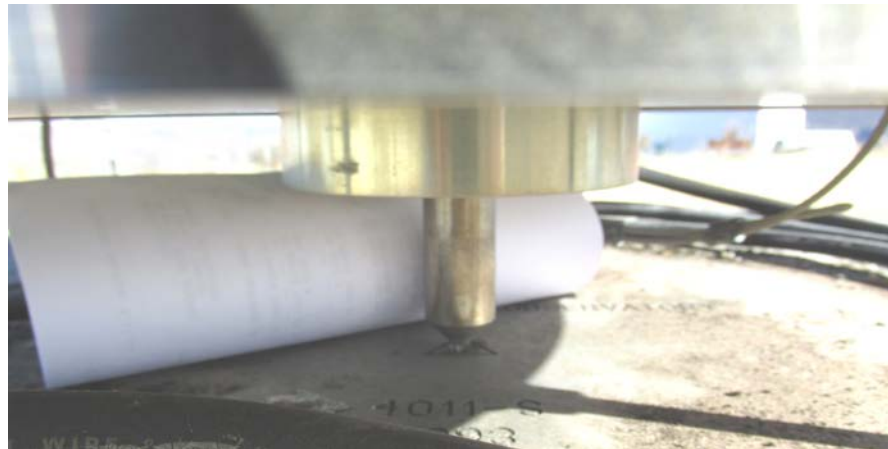
Figure 25 – Intersection observations to MDO1 and the ARP were made to the left and right side of the centering pin (left and right tangent observations) to determine the horizontal direction. Each set of left and right tangent observations are averaged together in lieu of a single observation to the center.
