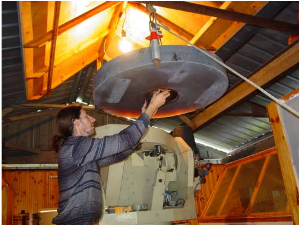
Figure 13-46. Replacement of Lviv telescope mirrors.
