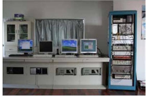
Figure 13-75. The control room of the Shanghai SLR station. The new pico-event timer (NPET) from Czech Technical University is shown in the middle of the rack; the timer was received in July 2009 and has a timing precision of 0.8ps.
