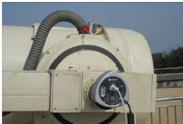
Figure 13-73. The Shanghai system's EMCCD camera, installed on the telescope.
