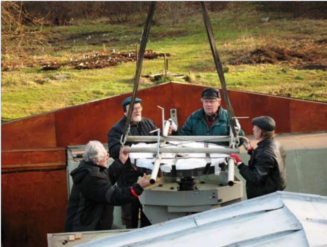
Figure 13-60. Recoated mirror before installation.
