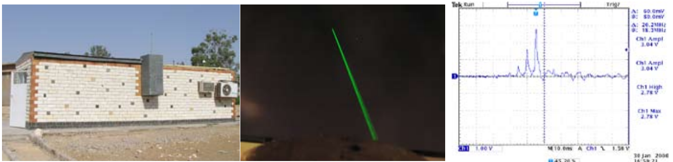
Figure 13-34 (a-c). External view of the Helwan station; satellite observations at night; the shape of the semi-train laser pulses, as measured by the oscilloscope.
