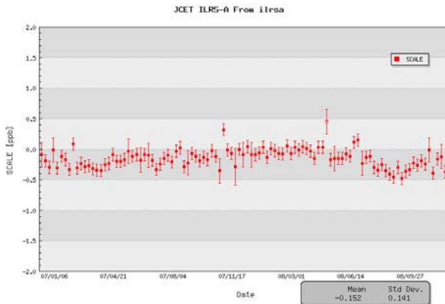
Figure 12-7. Time series of scale of the JCET weekly contribution with respect to the ILRS combination product for 2007-2008. The 0.141 ppb standard deviation corresponds to less than 1 mm in length.
