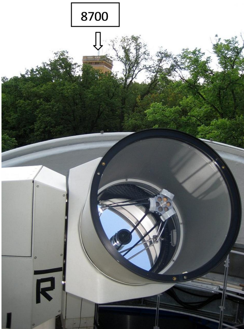
Figure 4 SLR 7841 receiver telescope and location of temporary marker 8700 on top of building A 62 in the background
