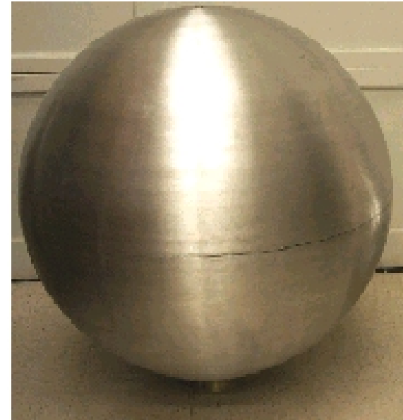
Starshine 3 sphere without mirrors or cubes
