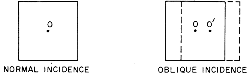
Figure 7. Displacement of the input and output apertures in the plane of the front face.
