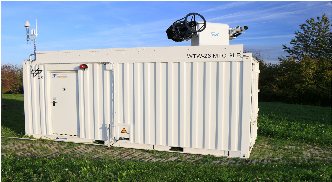
STAR-C, our transportable space debris laser ranging station © DLR
